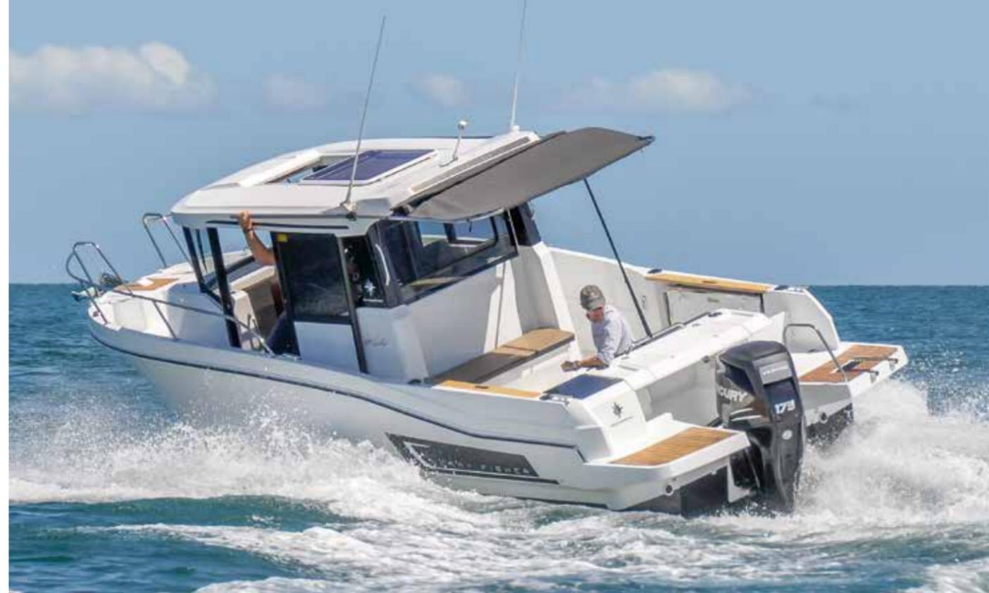
The transom combines great looks with functionality. There's a walk-through from the large transom platforms that sets the stage for water play. In the middle is a moulded table with refreshment holders, incorporating a flip-up cutting board to allow full engine tilt. On the port side is a nice big livebait tank, which I'm thinking could also double as a wine cooler.
