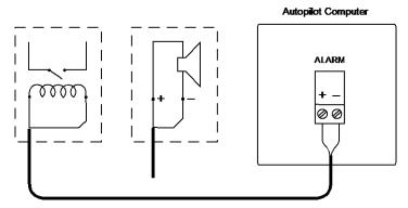
Figure 2-23 External alarm connection
