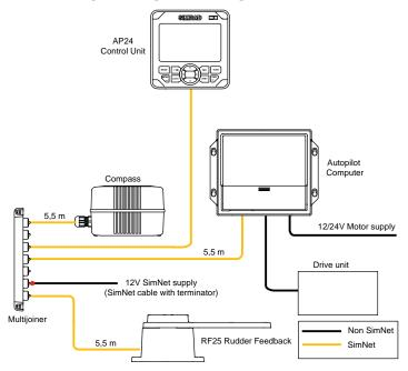
Figure 2-1 AP24 basic system layout
