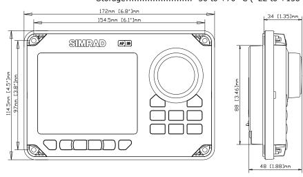
Figure 4-2 AP28 Control Unit – dimensions (Mounting bracket is optional equipment)
