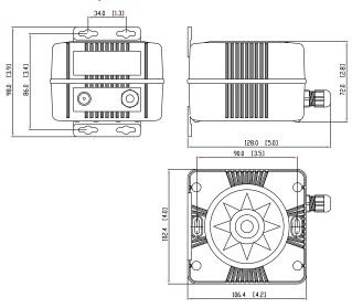
Figure 4-6 FC40 Fluxgate Compass - Dimensions
