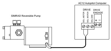
Figure 2-10 Connecting a reversible pump
