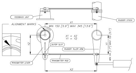
Figure 2-5 Rudder feedback mounting (019356)
