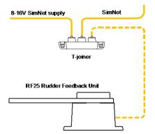
Figure 2-7 RF25 connection to SimNet
