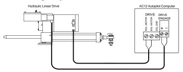
Figure 2-11 Connecting a hydraulic linear drive
