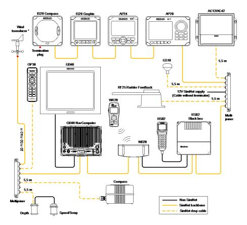
Figure 2-22 SimNet network, expanded system
