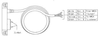
Data converted from SimNet/NMEA2000 to NMEA0183 (TX) and vice versa (RX).
