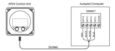
Figure 2-4 Control unit connection
