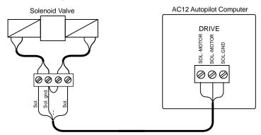
Figure 2-12 Connecting a solenoid valve
