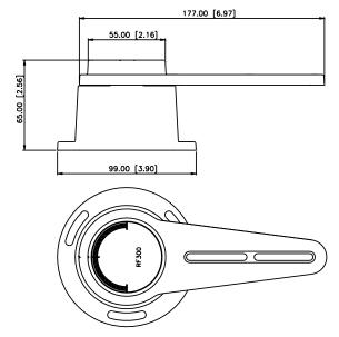
Figure 4-7 Rudder Feedback - Dimensions
