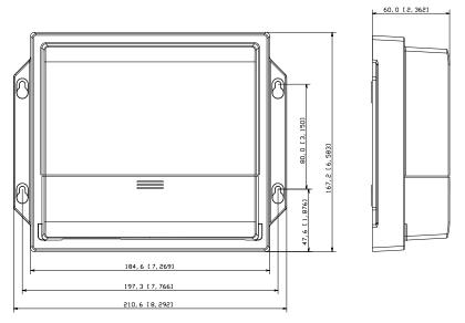
Figure 4-3 AC12 Autopilot Computer - Dimensions
