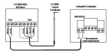
Figure 2-9 LF3000/LFI3000 Mk2 connections
