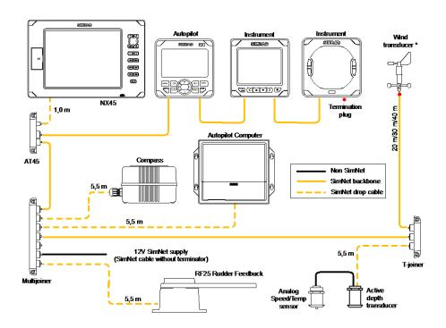
Figure 2-21 SimNet network, medium system
