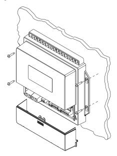
Figure 2-3 Autopilot computer mounting
