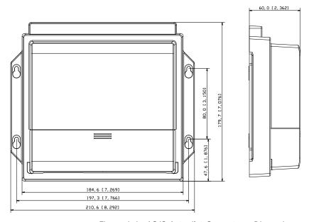
Figure 4-4 AC42 Autopilot Computer - Dimensions
