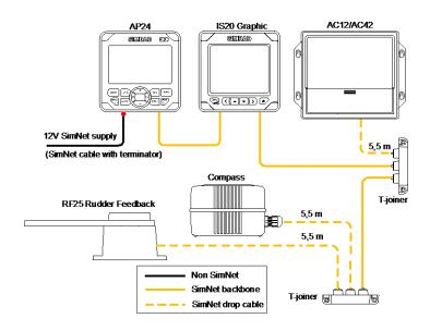
Figure 2-20 SimNet network, small system
