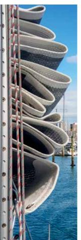
Mast and boom are aluminium by Sparcraft, with Dyform standing rigging. The backstay has a 24-purchase system adjustable in two speeds.
