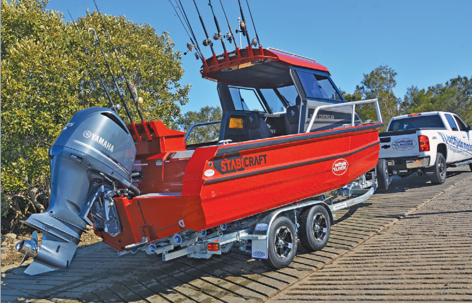
Above: Classic application of sheet aluminum in a trailerboat fishing environment: Tough, strong, seaworthy - and much lighter to tow than an equivalent GRP sportsfisherman - with more performance per given horsepower.
