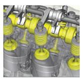
A compact, single-overhead-cam design and long piston stroke give Mercury 40 - 60hp FourStroke outboards more low-end torque for excellent acceleration, even when pushing a heavy load. The high-displacement, long-stroke, four-cylinder, single-overhead cam design provides optimum power and a smooth ride with Command Thrust models.
