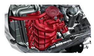
Compact and simple in design, uses a single throttle body and long intake runners to pack in more air to build torque. Top mounted for a more pleasing sound.
