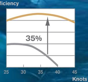
The forward-facing solution and an efficient flat-surface hull. The result is around 35% better efficiency at cruising than inboard shafts.
