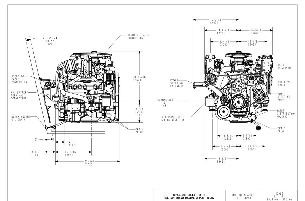
NOTES: (1) DIMENSIONS REQUIRE A MINIMUM OF 1/2 in. (13 mm) CLEARANCE FOR MOTOR MOUNT DEFLECTION.
